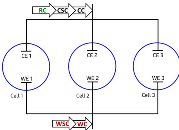
**Figure 2.** Schematic for connecting multiple channels to cells in parallel. It is not possible to find current flowing through each cell by running them in potentiostatic mode because current from one cell will try to flow through the other cell. (WE: working electrode, CE: counter electrode, RE: reference electrode, WSC: working electrode sense clip, WC: working electrode clip, RC: reference electrode clip, CSC: counter electrode sense clip, and CC: counter electrode clip)
