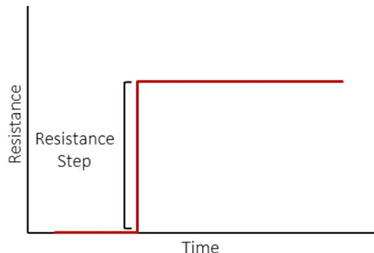
**Load resistance:** The Squidstat discharges an electrochemical device at this resistance. The set value for resistance should be positive.
